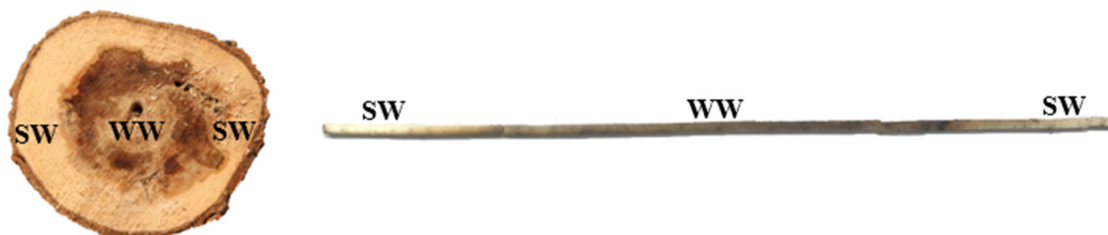
Figure 1. Sample collection by dividing wood tissues into two parts: (1) SW: sapwood, located in the outer edge of trunk with normal white color; (2) WW: wetwood, located in the central zone of trunk with brown color.
